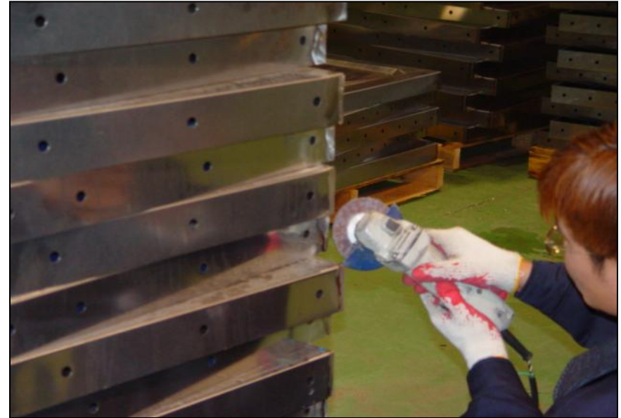
Welding Portion it Trims -2
